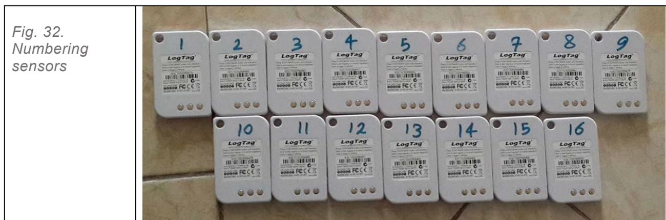
If you are mapping temperature in very large cold rooms (e.g. drive-in cold rooms) up to 40 sensors are required. Do not forget the extra sensor for recording ambient temperature.
