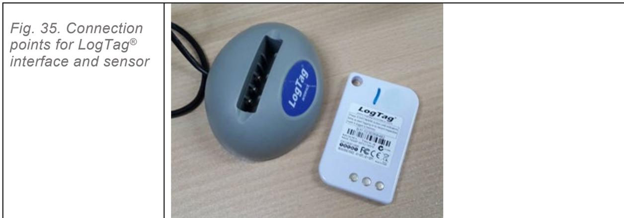
*Fig. 35. Connection points for LogTag® interface and sensor*
